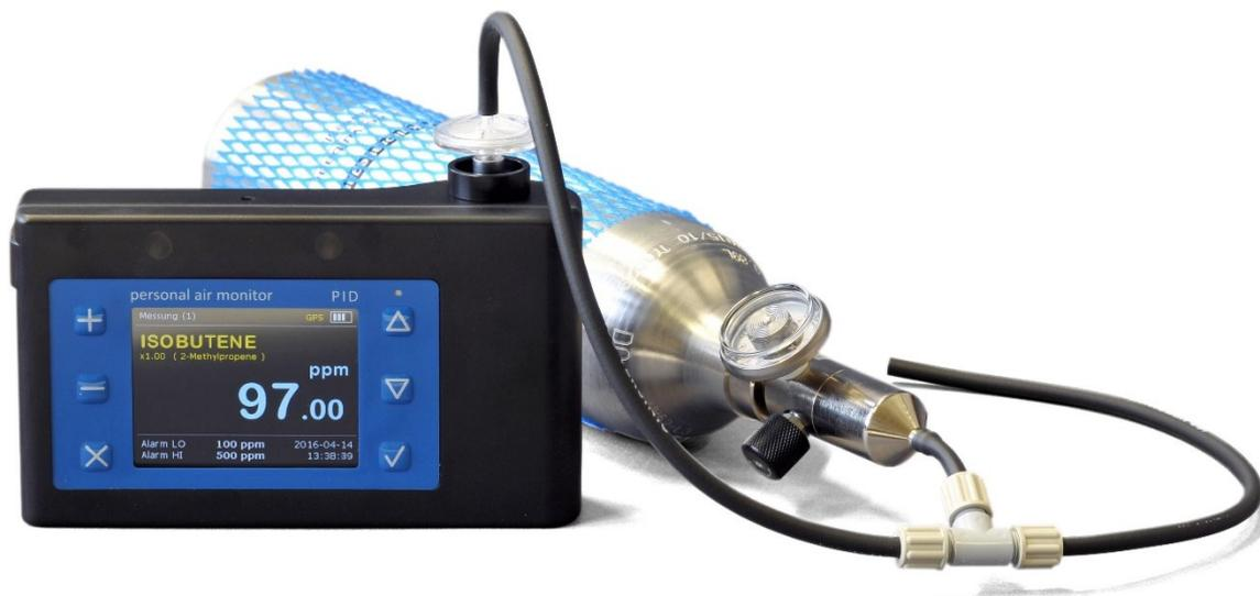
Figure 10 Calibration assembly
